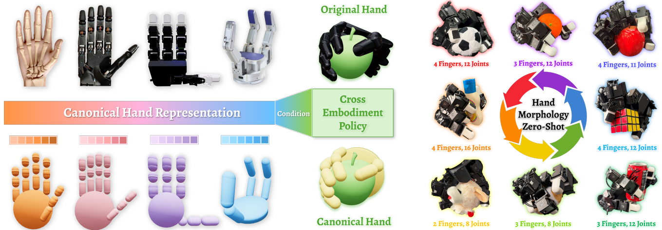
Fig. 1: We introduce a canonical hand representation that unifies diverse dexterous hands into a shared parameter space and canonical URDF format, serving as a condition for cross-embodiment policy learning. It enables dexterous grasping and zero-shot generalization to novel hand morphologies, highlighting its potential for a wide range of dexterous manipulation tasks.
